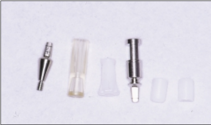
Figure 7: Michael used Astra's new Direct Abutment to restore his father's lower incisor. The components are supplied in kit form as shown here (Left to right: the solid titanium Direct Abutment, the plastic abutment carrier, the impression pick-up coping, laboratory analogue and two healing caps. The kit includes one healing cap for temporisation and another to be used for laboratory wax-up/burn-out
